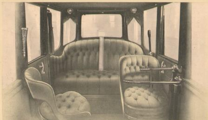
This view of Model 60 illustrates the Detroit Duplex Drive. Observe that when one set of operating levers is in driving position, the other set must be folded against side of car.
